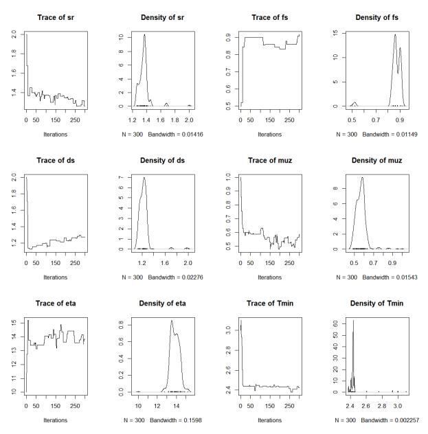
From the traceplot we can see that with only 300 iterations the chains have neither mixed well, nor reached stationarity. For demonstration purposes we remove a burnin period of 100 samples and have a look at parameter correlations, and the overlap between the posterior and prior densities.
